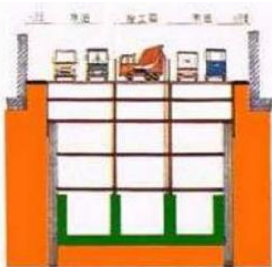
4. Construction of main structure (down - up)
