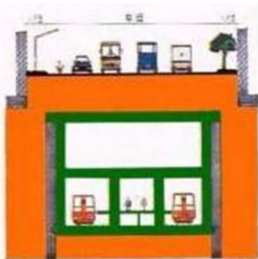
6. Completion of underground station
